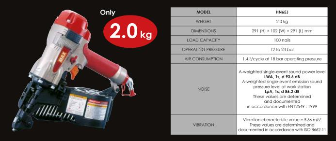
HN65J is our 65 mm Powerlite coil nailer for fastening metal joints in wooden structures. It has a part that can be used to find a hole, making your work easier since you do not need to aim for a hole – the tool does it for you. It has a depth adjustment dial, movable swivel joint, and special end cap that the tool can clean by itself. HN65J is compact, but you can load 100 nails into the magazine so that you can work in narrow spaces.
